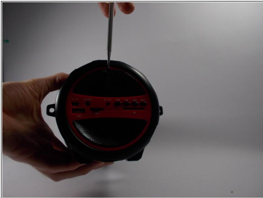
**i** If there are no signs of wire damage in these locations, then it's time to remove the red interface plate.
