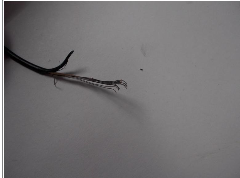
**i** Faulty wires can usually be located by spotting physical damage to the wire itself such as: fraying, complete disconnection, or a notched appearance.
