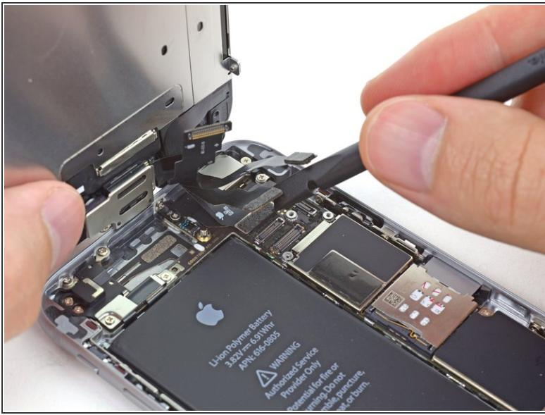
! Make sure the battery is disconnected before you disconnect or reconnect the cable in this step.
