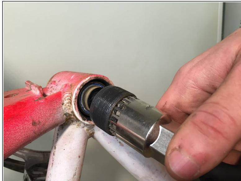
*(i)* Go to the side that does not have the drive train. This side must be completed first!
