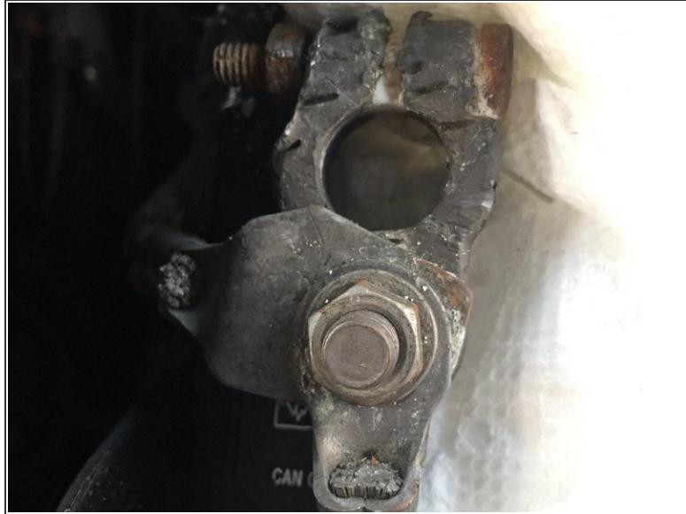
**⚠ Always remember to remove the negative terminal first before the positive terminal. This will prevent shorting to the ground and possibly causing shock or a fire.**
