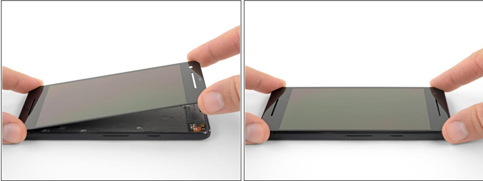
*(i)* In this step, you will temporarily install the new screen in order to properly align it with the front-facing camera bracket while adhering the bracket to the screen.
