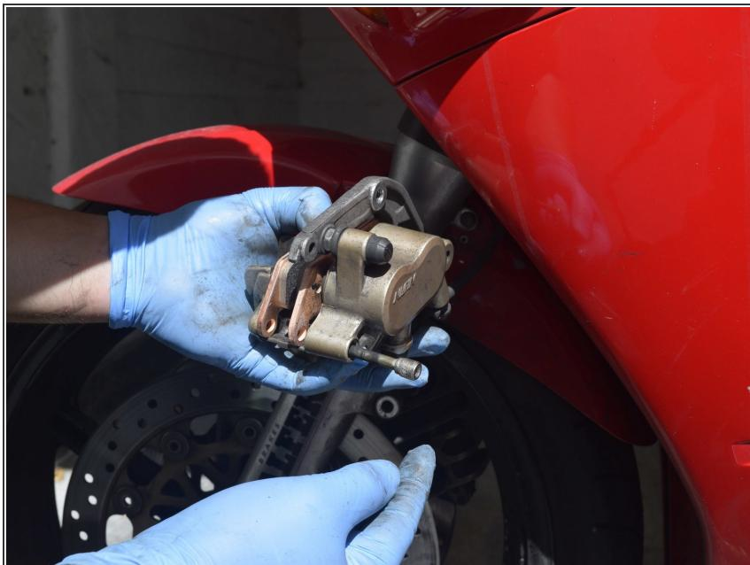
*i* If you haven't cleaned the retainer pin with soap and water, now is a good time. If any corrosion is present on the smooth part of the pin, use steel wool to smooth it out. If you have brake grease available, you can apply a thin coat to the smooth part of the pin.
