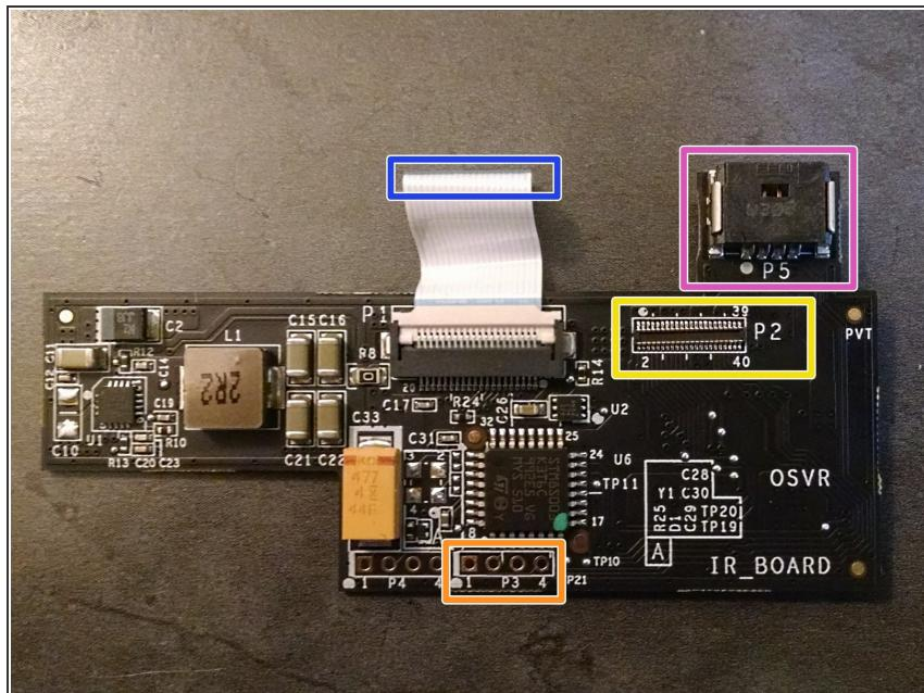
ⓘ This is a view of a HDK v1.4 and up IR board, looking at the side that faces the outside of the HMD. When re-installed, the left edge of the board as seen here goes toward the top of the HMD.
