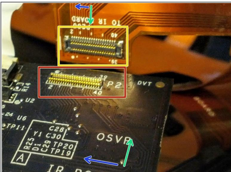
**(i)** This LED ribbon cable to IR board connection can be intimidating at first, because it feels "directly connected" to the board - but it's actually just a connector on the IR board face. The first two images are from a teardown of a modified 1.2 (you'll never see it like this in your own device) but they'll give a better idea of how it's connected.
