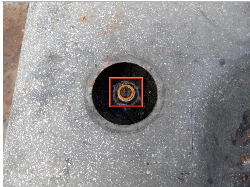
⚠ If the screw threads do not rise above the locking nut then **STOP**: The steering box is worn out, it is time to rebuild it, or replace it! Failure to do so could result in your steering system failing.
