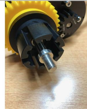
① Add wheel spacer on axle which helps to keep tension between bearings
