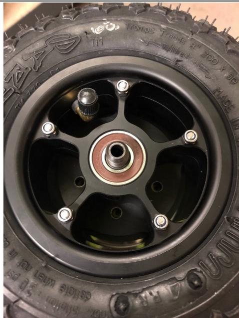
⚠️ Make sure 5 x M4 bolts are tighten securely.
