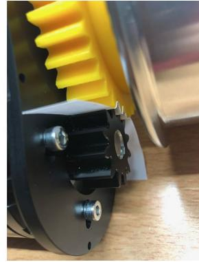
**⚠** Baseplate should be parallel to the wheel otherwise wheels will mesh on angle and will cause negative effects.
