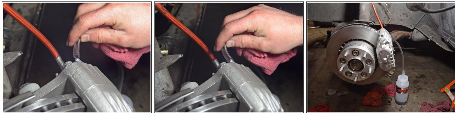
① Begin the bleeding procedure at the driver side rear brake caliper.
