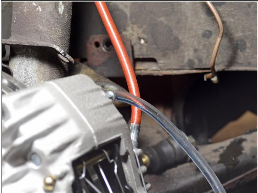
**i** If there is still fluid left in the tank after bleeding all four corners of the car, you will need to keep the bleed tube on the passenger front bleed valve.
