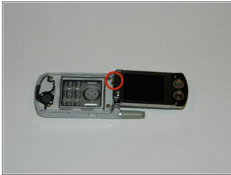
**⚠** The fragile wire strip connecting the display housing to the circuit board is located on the left side of the inner hinge.
