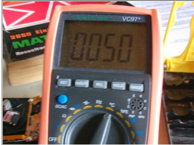
ⓘ I used a multimeter with temperature measurement; it's not exact but it works.
