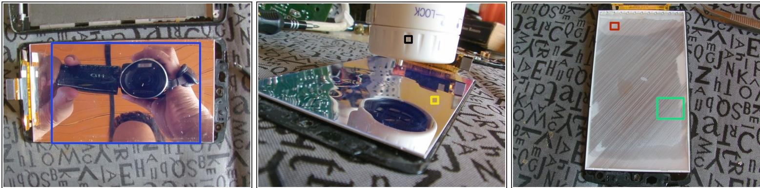
ⓘ I used a hair dryer with cold air to help to separate the layers.
