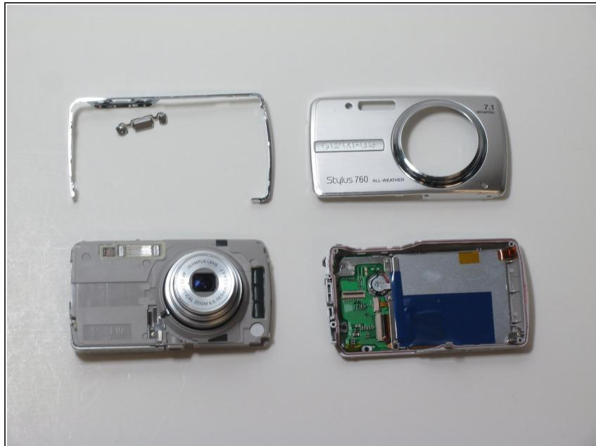
*(i)* You should be left with 4 large pieces, the outer case, inner lens piece, outer silver band and back case containing the LCD display.
