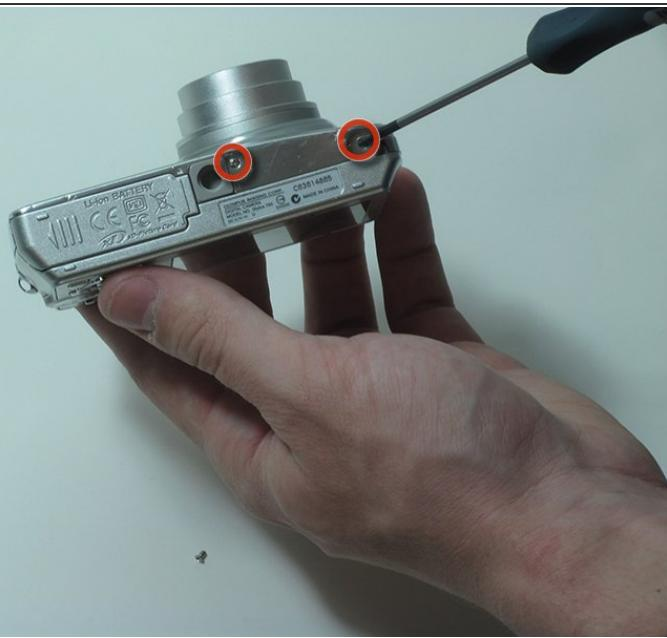
⚠ Before starting, be sure to remove the battery from the camera. See [Removing the Olympus Stylus 760 Battery Guide](#) for details.
