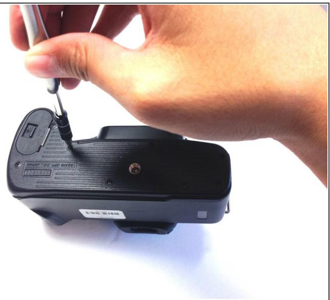
*(i)* Place the lens face up to locate the bottom cover.
