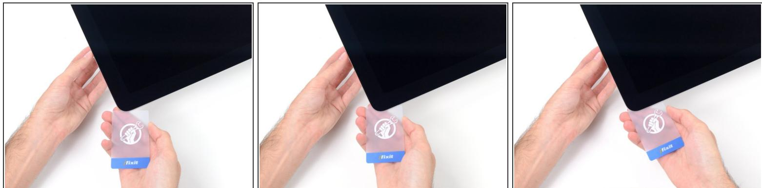
**i** While the opening tool did the lion's share of the work, the display will still be slightly adhered to the case. A plastic card will be necessary to free up the last of this adhesive.
