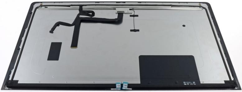
**i** If you are replacing the display panel, you may need to transfer additional components from the old panel to the new one. Compare the back of the old display with the replacement display. Note all cables, sensors, and foam cushioning that are missing from the new display.
