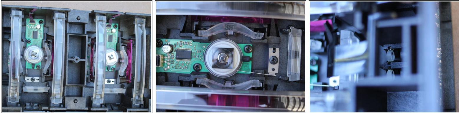
**⚠** These are lenses, mirrors, and sensors used by the printer to determine how it is printing. Any damage will affect the quality of printing.
