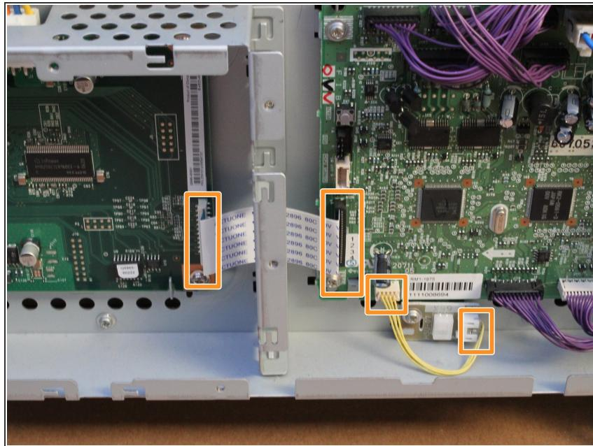
*(i)* During the next two steps, do not unplug any of the connections in the example boxed in orange.
