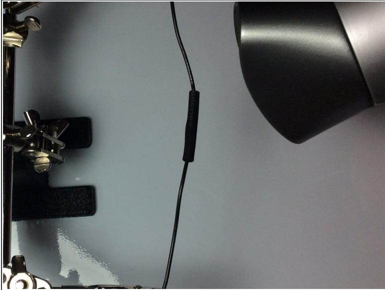
*(i)* To properly protect the soldered wire connection, use heat shrink.
