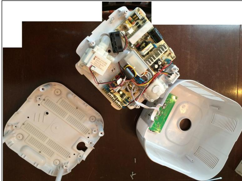
! Flip cube over (carefully supporting the inside mechanism--its not attached to the case anymore) and then lift case off. Don't go yanking it away brusquely, that control cable may have gotten pinned underneath even though you disconnected it.
