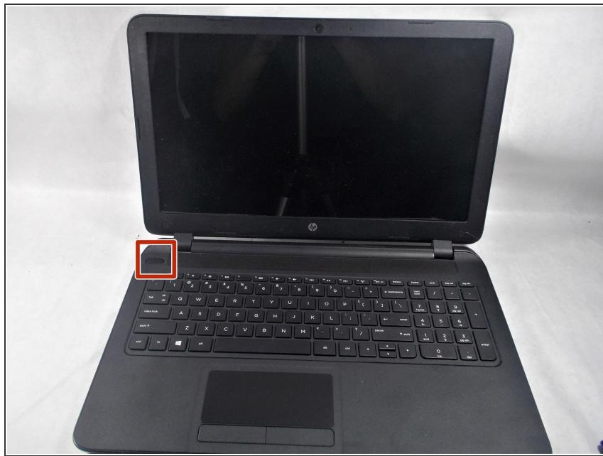
! Turn off the computer. If you are unsure whether the computer is off or in Hibernation, turn the computer on, and then shut it down through the operating system.
