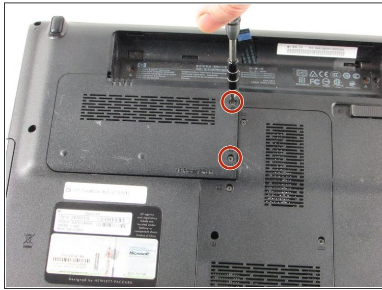
**⚠** Shutdown your computer and remove the battery before beginning the replacement.
