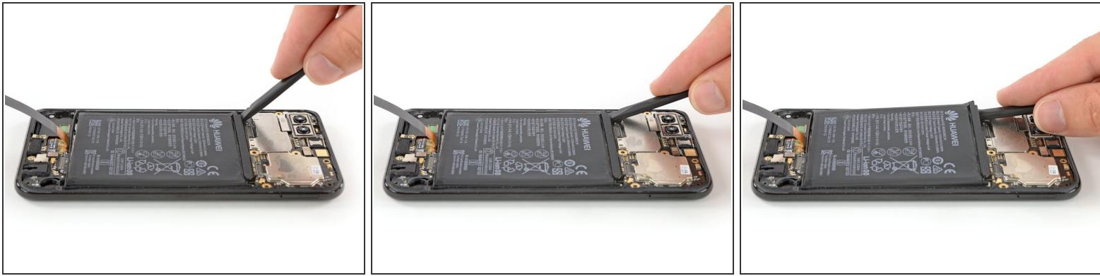
*(i)* If you have trouble prying up the battery, the adhesive may not be loose enough. You can apply some isopropyl alcohol under each corner of the battery and allow it to penetrate for several minutes to help weaken the adhesive.
