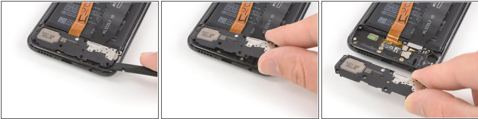
ⓘ There's a little bit of adhesive under the loudspeaker. It's possible to remove the loudspeaker without heating the adhesive but if you're having a hard time removing it, you can [use an iOpener](#) to soften the adhesive.
