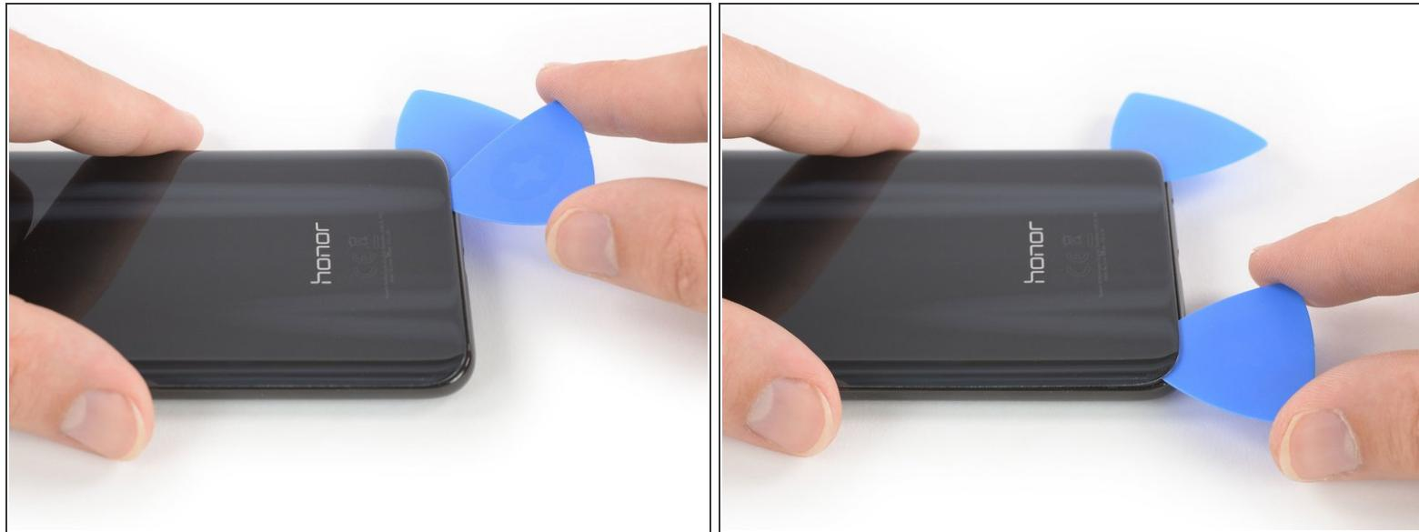
*(i)* **Apply more heat** if the adhesive becomes hard to cut. During the removal process, the back cover is under tension all the time and is likely to break if the adhesive isn't softened enough.
