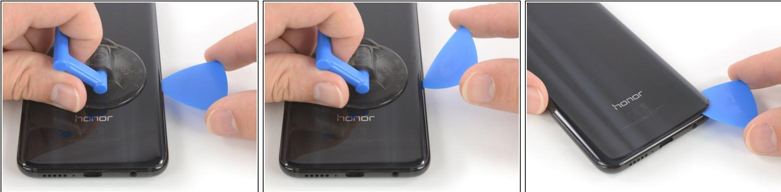
ⓘ If the phone's rear glass is cracked, the suction cup may not stick. Try [lifting it with strong tape](#), or superglue the suction cup in place and allow it to cure so you can proceed.
