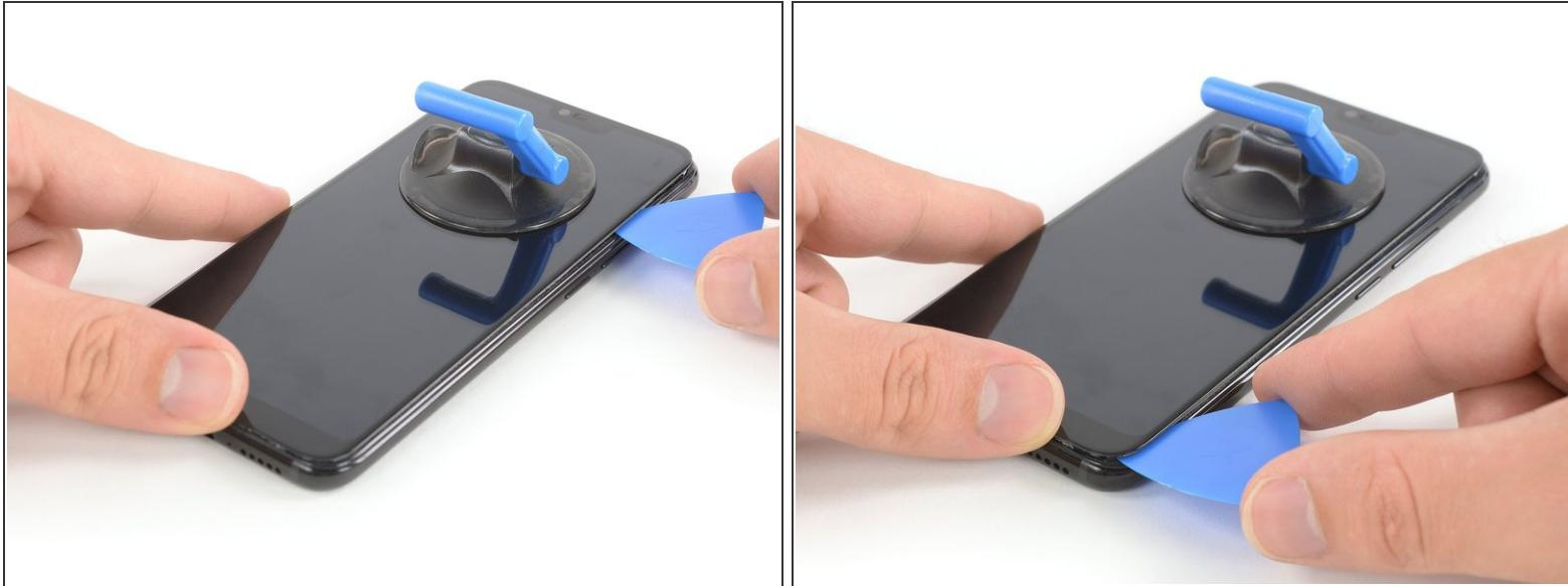
⚠ While cutting, make sure the pick slides **under the display panel** and not just between the display and the front glass.
