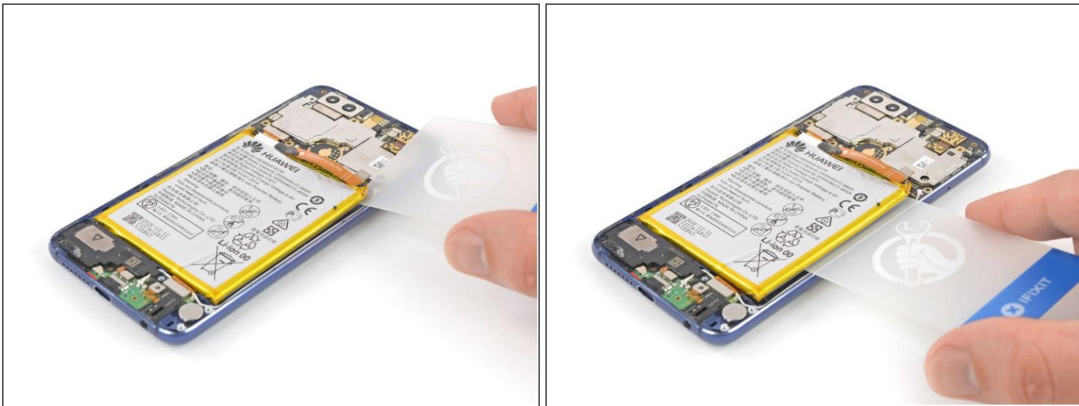
**⚠** Try to deform the battery as little as possible during the following process. Soft-shell lithium-ion batteries can leak dangerous chemicals, catch fire, or even explode if damaged. Do not use excessive force or pry at the battery with metal tools.
