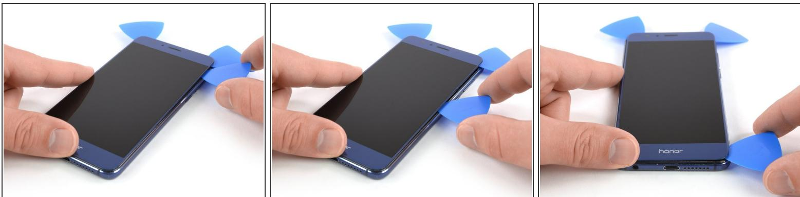
! While cutting, make sure the pick slides **under the display panel** and not just between the display and the front glass.
