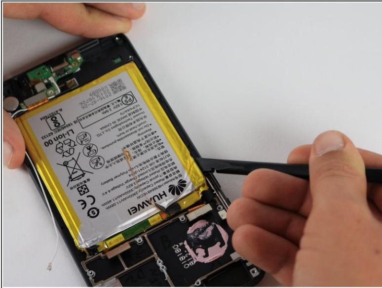
**⚠** Avoid using a heat gun for this step as overheating the battery can cause permanent damage.
