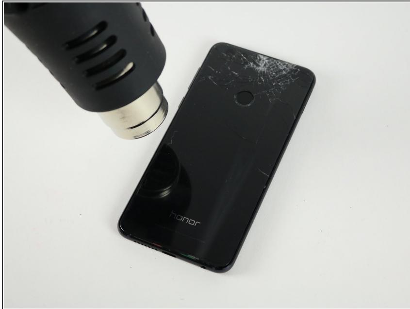
**⚠** Make sure you spend at least 5 minutes heating up the adhesive. Prying off the glass cover too early can result in cracking the panel.
