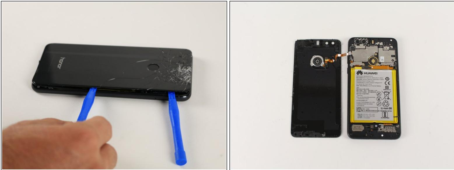
**⚠** Be careful not to tear the orange ribbon wire when removing the back panel.
