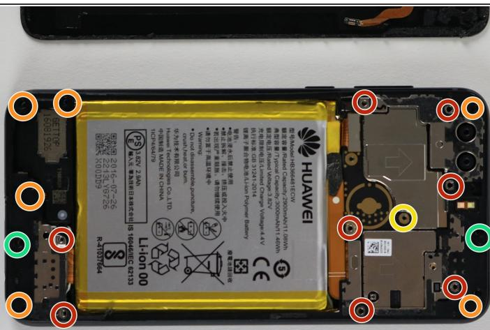
**i** Keep the tiny screws on a magnetic pad or a designated area so they will not be lost. There are eighteen screws in total.
