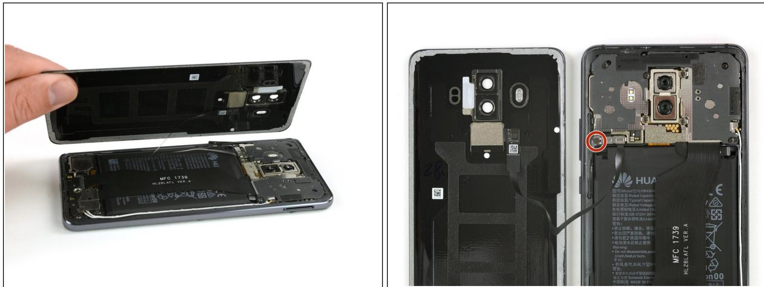
**⚠** Don't remove the back cover all the way, yet. The fingerprint sensor cable is still connected to motherboard.
