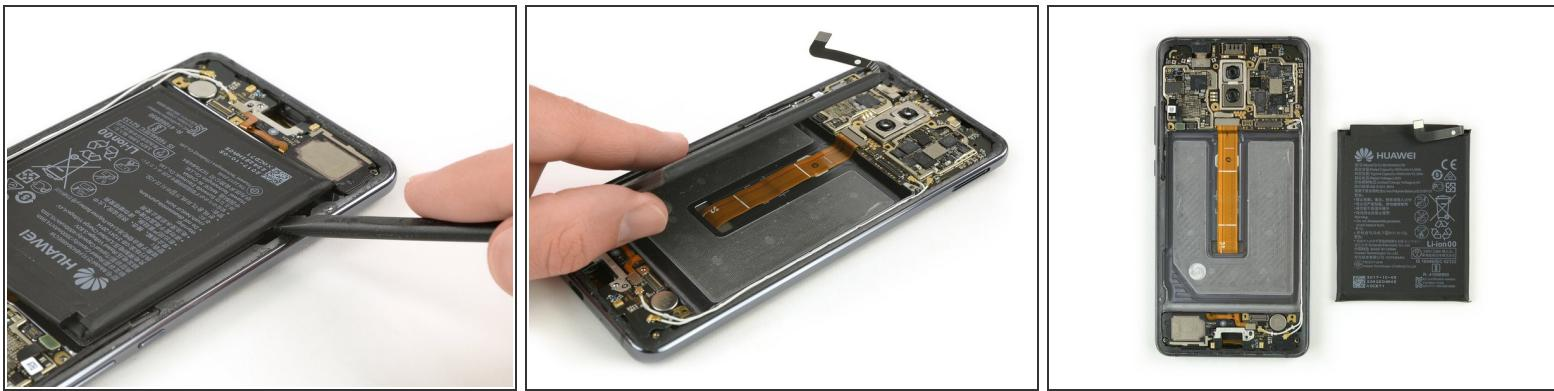
**⚠** The display flex cable runs underneath the battery. So be careful not to damage it when loosening the adhesive. Also take care not to bend or puncture the battery at any time.
