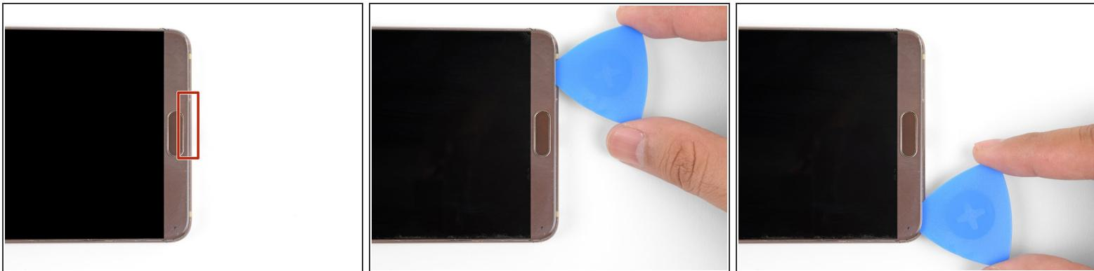
! As you slice through the bottom edge, be careful not to slice near the right edge of the fingerprint sensor. It contains the sensor ribbon, which is prone to damage.
