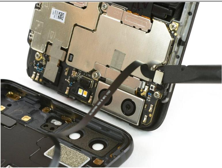
**⚠** Don't open the phone all the way, yet. The cable for the standby and volume buttons is still connected to the back cover.
