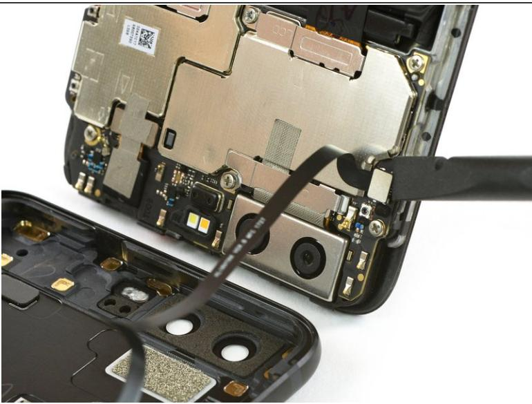
! Don't open the phone all the way, yet. The cable for the standby and volume buttons is still connected to the back cover.
