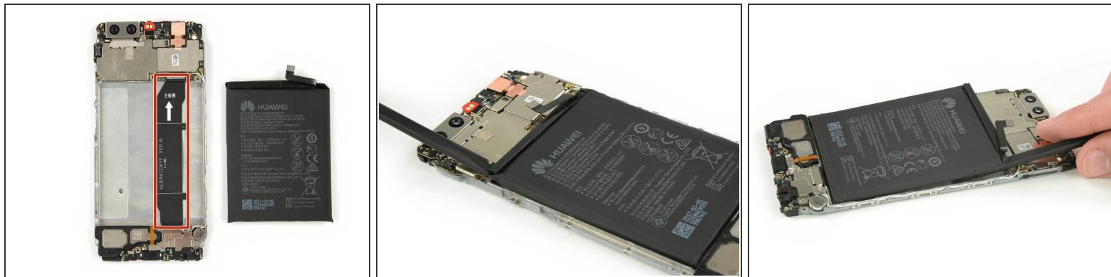
**⚠** In the following steps it is important to avoid bending or puncturing the battery, damage can result in battery fire.
