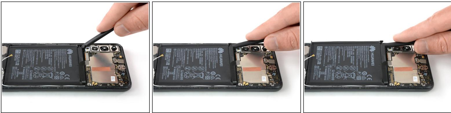
**i** In case you have trouble to pry up the battery the adhesive may not be loose enough. You can apply some isopropyl alcohol under each corner of the battery and allow it to penetrate for about two minutes to help weaken the adhesive.
