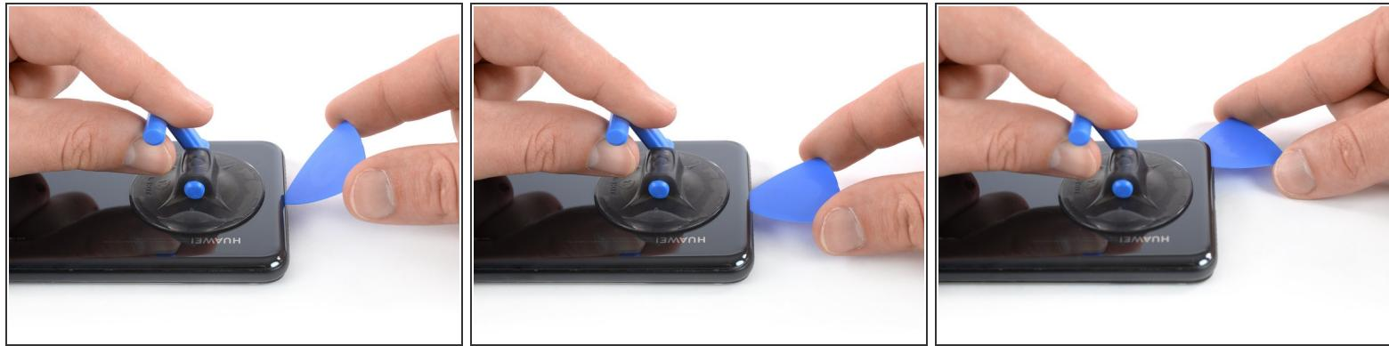
**i** If the phone's rear glass is cracked, a suction cup may not stick very well. Try [lifting it with strong tape](#), or superglue the suction cup in place and allow it to cure so you can proceed.
