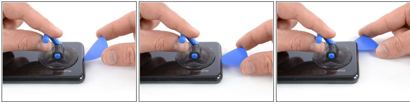
ⓘ If the phone's rear glass is cracked, a suction cup may not stick very well. Try [lifting it with strong tape](#), or superglue the suction cup in place and allow it to cure so you can proceed.
