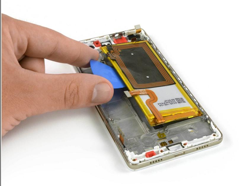
**⚠** To avoid thermal runaway, including fire, do not bend or puncture the battery
