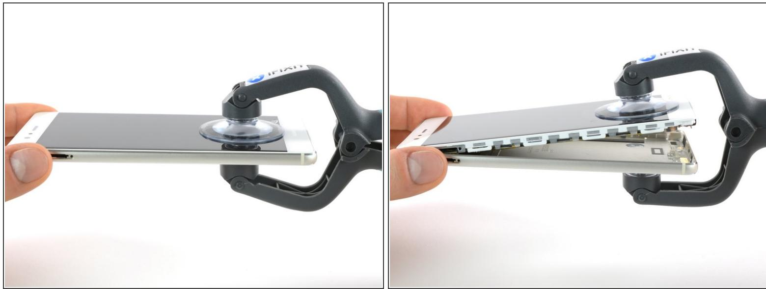
**⚠** Avoid to lift only the display instead of the whole phone assembly as doing so may cause damage to the screen.
