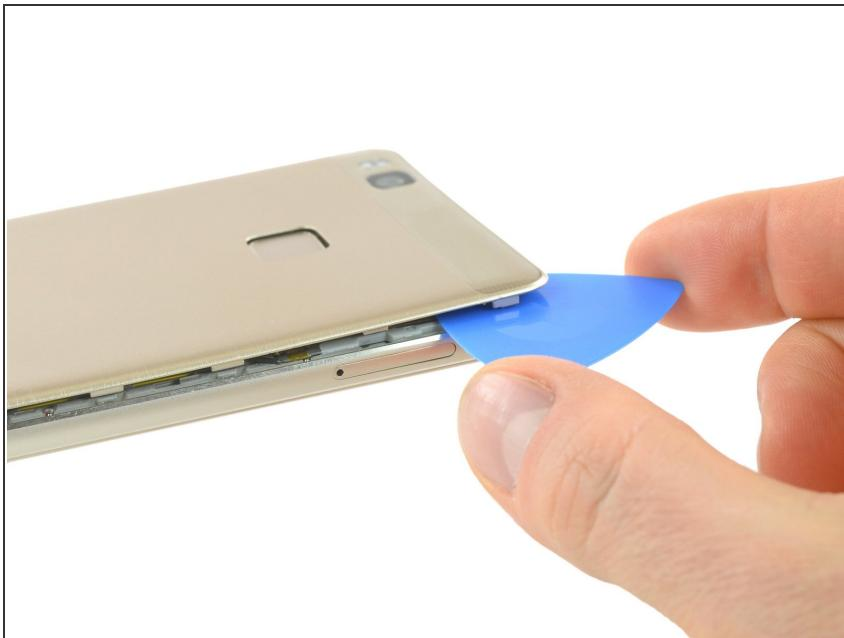
*ⓘ* There is adhesive underneath the back cover that holds it to the battery and the metal plate at the top.
