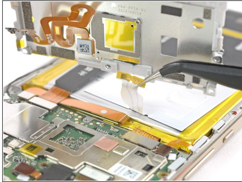
! Do not remove the shield plate yet, it is attached by a connector and an adhered cable.
