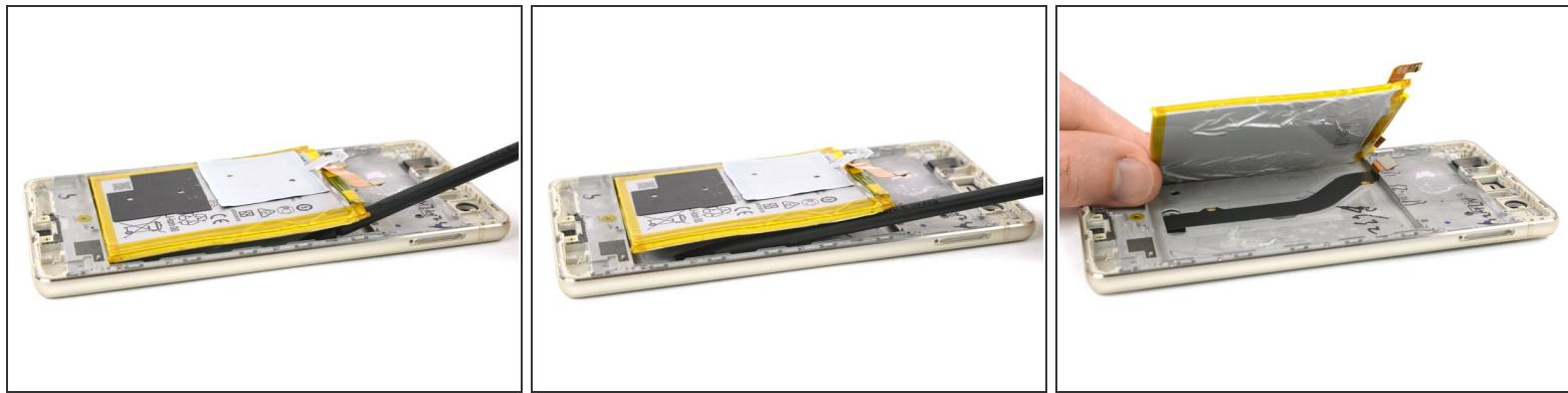
**⚠** Only pry along the SIM tray edge of the battery to protect the display flex cable that runs under the center of the battery.
