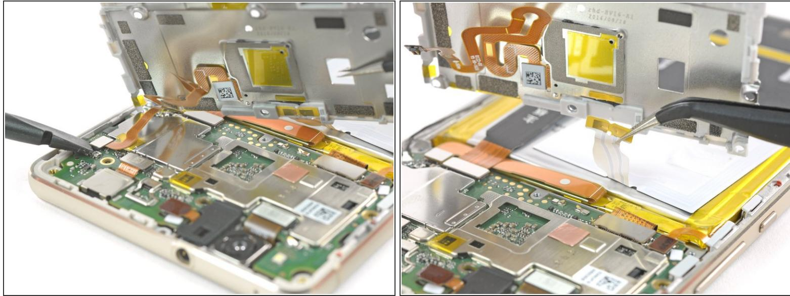
⚠ Do not remove the shield plate yet, it is attached by a connector and an adhered cable.
