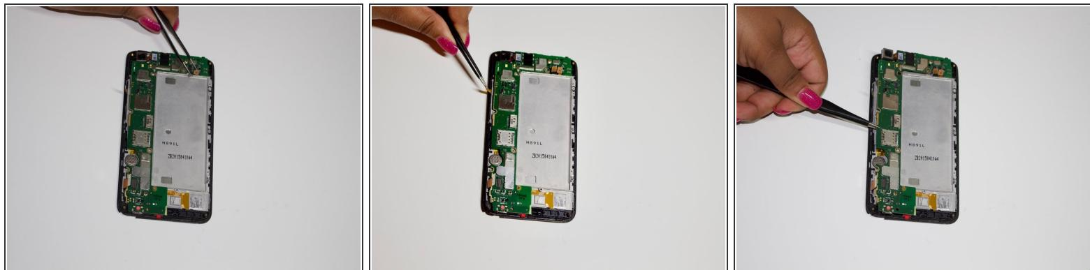
! Ensure that all latches are detached and that there are no extra screws to avoid damaging the motherboard.
