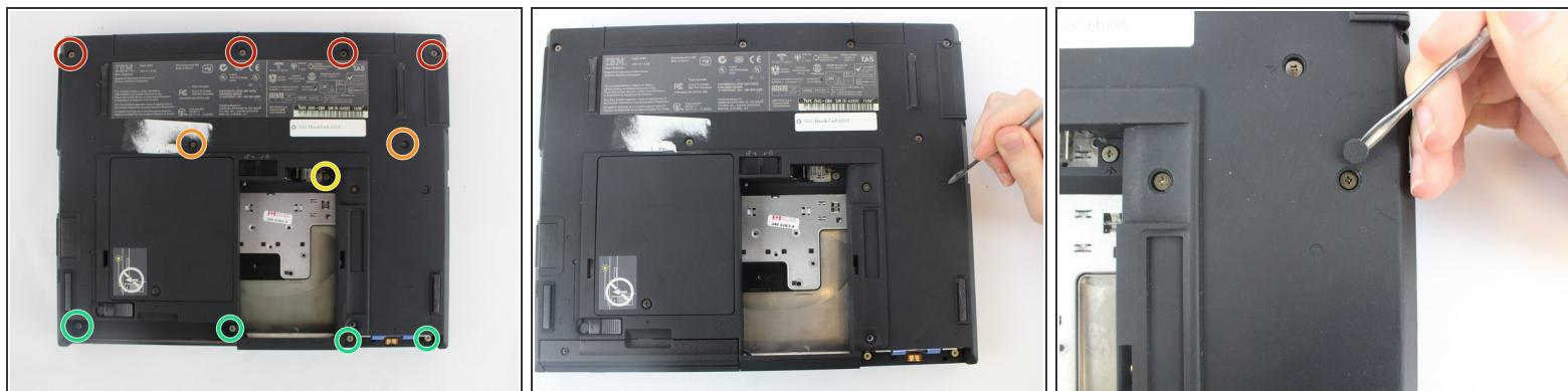
*(i)* Most of the screws have a small, plastic covering attached with an adhesive. Use the metal spudger to pry it off. Make sure to note which screw came from which hole.
