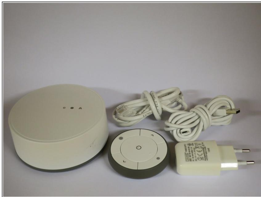
*(i)* The Gateway I'm tearing down today came from the Ikea Gateway Kit, which includes the Gateway, two bulbs, a remote, a USB A to Micro-B cable, a Ethernet cable and a 5V @ 1A charger.
