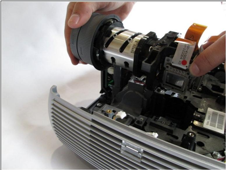
*(i)* Carefully hold the lens from both ends and lift up simultaneously
