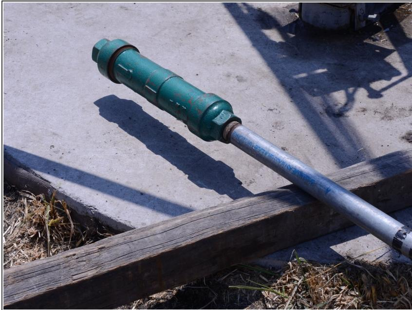
*i* The last section of riser main pipe will have the pump cylinder attached to the bottom.
