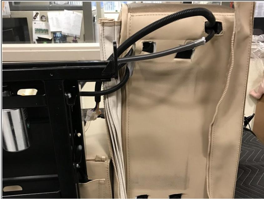
⚠️ Upper piece will still be connected to the lower half via Wire harness and air hose be careful NOT to Drop or Pull on these as it may require you to disassemble even further in order to fix.
