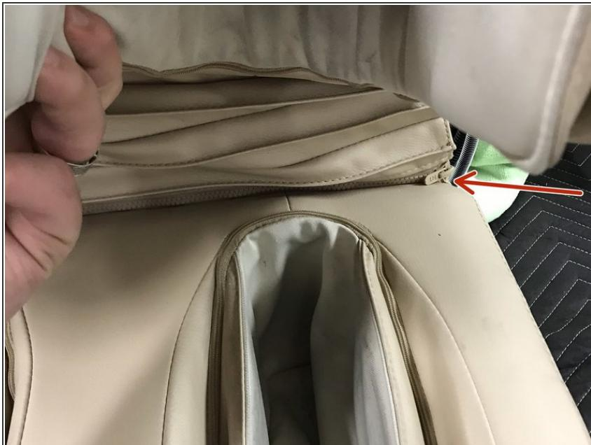
*(i)* Lift up on the Upper portion of the footrest and unzip the leather in the middle. This will separate the upper from the lower.
