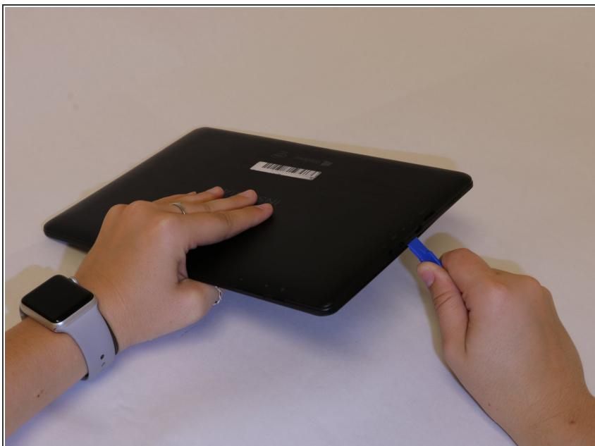
● Lay the screen flat on its surface and use the iFixit opening tool to remove the cover by gently prying the back cover from the screen.
