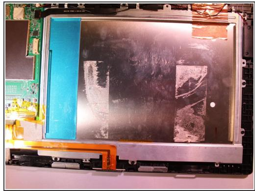
**⚠** Make sure not to bend the battery too excessively as if bent too much, it could rupture a cell within the battery and possibly cause a fire.
